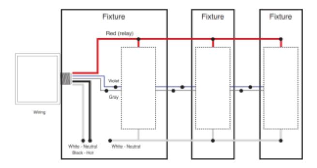
The maximum number of Fixtures can not exceed Sinking Current (100mA) based on dimming control.
