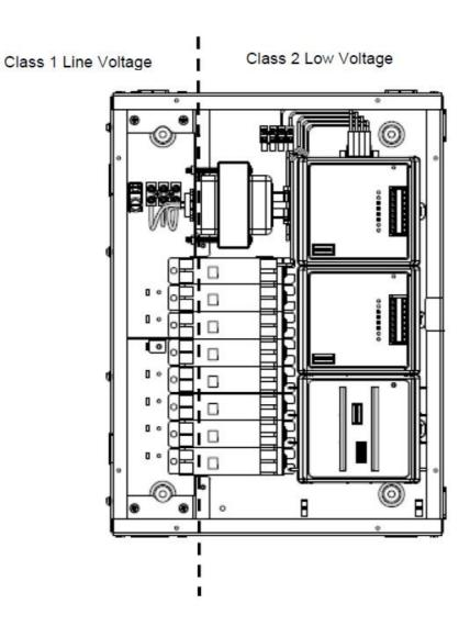
If there are different load voltages are used (120VAC/277VAC or 120VAC/347VAC), install the included barrier plate between the appropriate relays to create separate voltage compartments.
