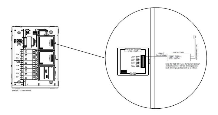
Connect Dialog network devices and expansion panels to main panel
