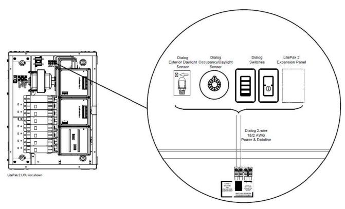
NOTE: Network connection to terminal block dependant on number of peripheral devices and expansion panels. Less than 15 use left two positions. 15 or greater, use right 2 positions
