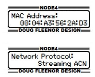
To view the **Medium Access Control Address** (MAC Address), press the **NET** select key. This will display the network settings menu. Press the **DOWN** arrow key three times to display the MAC Address page. This value is not configurable.
