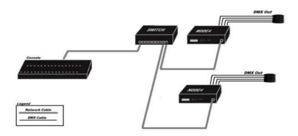
A typical network system will contain at least one console, one or more NODE4s, and an Ethernet switch. In the system shown above, the console is connected by an Ethernet cable to an Ethernet switch. An Ethernet cable is connected from the switch to each NODE4. Category 5e or higher cabling is required for 100Mbs operation in an Ethernet network.
