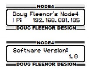
The **HOME** page shows the unit's name and current IP address. This is the default screen at startup, and you can return to it at any time by pressing the **BACK** key until you reach the HOME screen. Pressing the DOWN key from this page will display the Software Version page.
