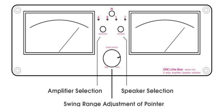
The long Press Button of Amplifier Selection can Power VU3 ON or OFF
