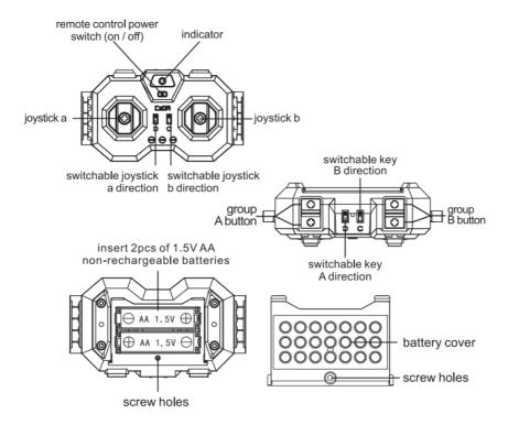
insert 2pcs of 1.5V AA non-rechargeable batteries according to the correct polarity of the battery (not included, should purchase separately)
