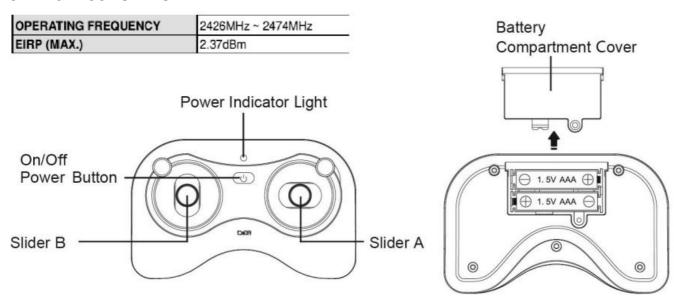
Install 2 pcs of 1.5V AAA nonrechargeable batteries in the correct polarity (remote control batteries are not included.
