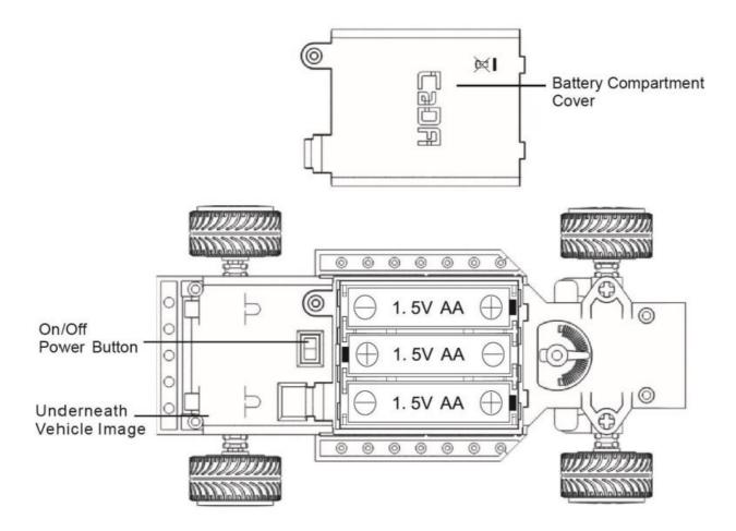
Install 3 pcs of 1.5V A nonrechargeable batteries in the correct polarity (vehicle batteries are not included).
