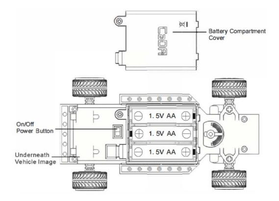
Install 3 pcs of 1.5V AA non rechargeable batteries in the correct polarity (vehicle batteries are not included).
