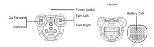
Insert 2 pcs of 1.5V AA non-rechargeable battery as per the correct polarity. Batteries are not included.
