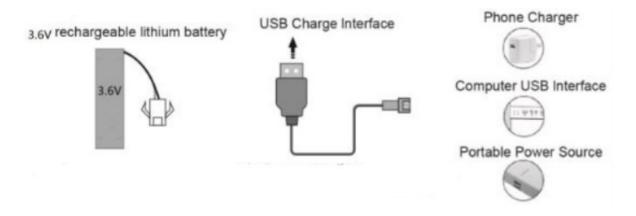
Insert 1 pc of 3.6V rechargeable lithium battery as per correct polarity Charge the rechargeable battery charging line included in this product.
