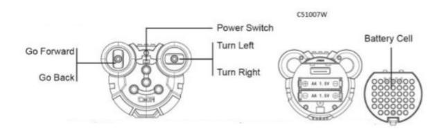
Insert 2 pcs of 1.5V AA non-rechargeble battery as per the correct polarity. (Batteries are not included.)
