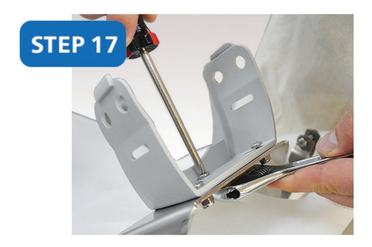
Attach the Dosatron bracket to the cart using the screws included on the cart. Using a Phillips head screw driver and a box or crescent wrench, tighten the screws.
