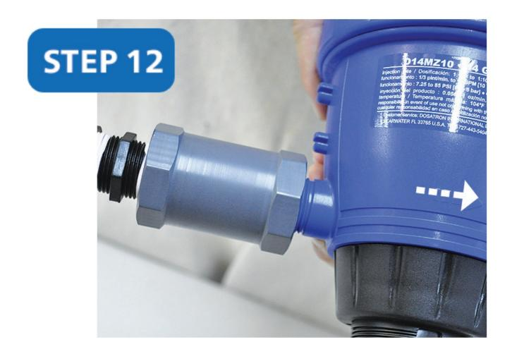
Pick up your inlet assembly and attach the flow restrictor end to the inlet side of the Dosatron. Note the direction of the arrow. Hand tighten.
