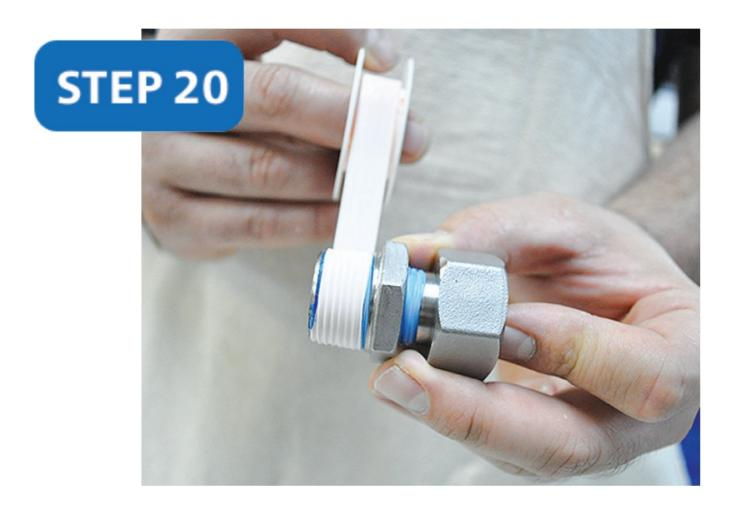
Wrap thread seal tape around the threads of the stainless steel hose adapter supplied with the cart
