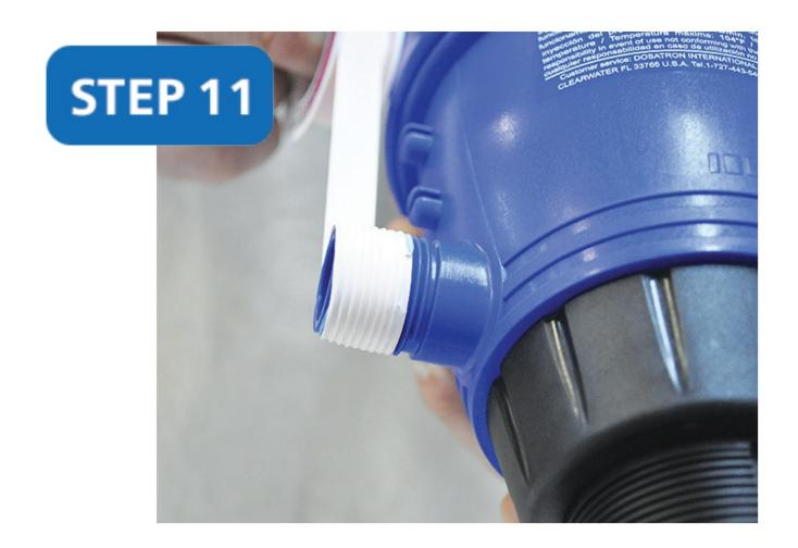
Before installing the assemblies, thread the inlet and outlet of the Dosatron with thread seal tape.
