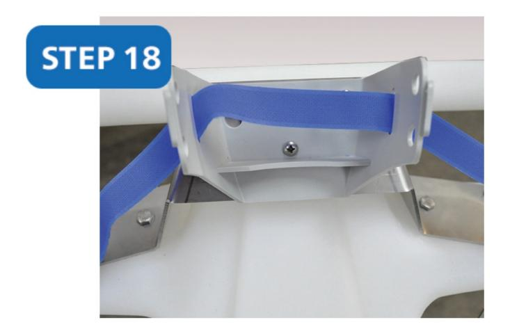
Thread the strap through the slits in the bracket.
