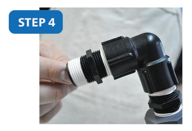
Attach the other 2" nipple to the other side of the elbow.
