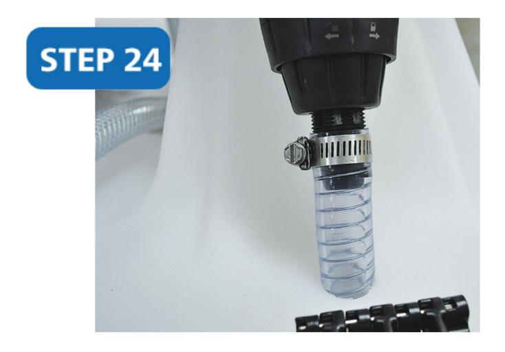
To attach the injection pickup hose to the Dosatron, place the strainer onto the hose and drop into the top of the cart tank. Thread the hose up through the hole on the top and attach a clamp to the hose. Thread the hose and clamp onto the Dosatron barb. Tighten clamp with a flat head screwdriver.
