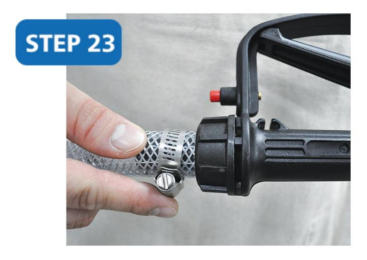
Place the hose clamp over the other end of the hose and attach to the gas style nozzle. Tighten the hose clamp with flat head screwdriver.
