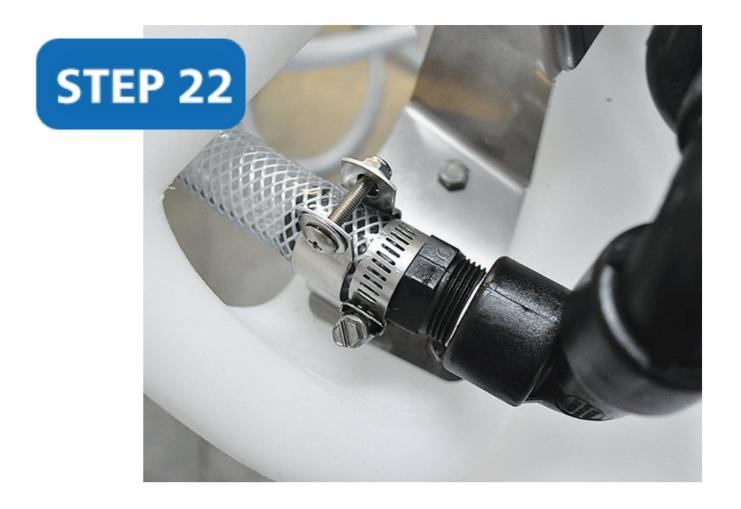
Install the stainless steel adapter parts by placing one washer on the inside of the cart bracket and one on the outside. Thread the stainless steel hose adapter onto the elbow and tighten with a box crescent wrench for a snug fit.
