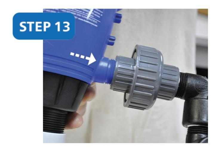
Pick up the outlet assembly and attach the union to the outlet side of the Decatron. Note the direction of the arrow. Hand tighten. You have completed installing both assemblies.
