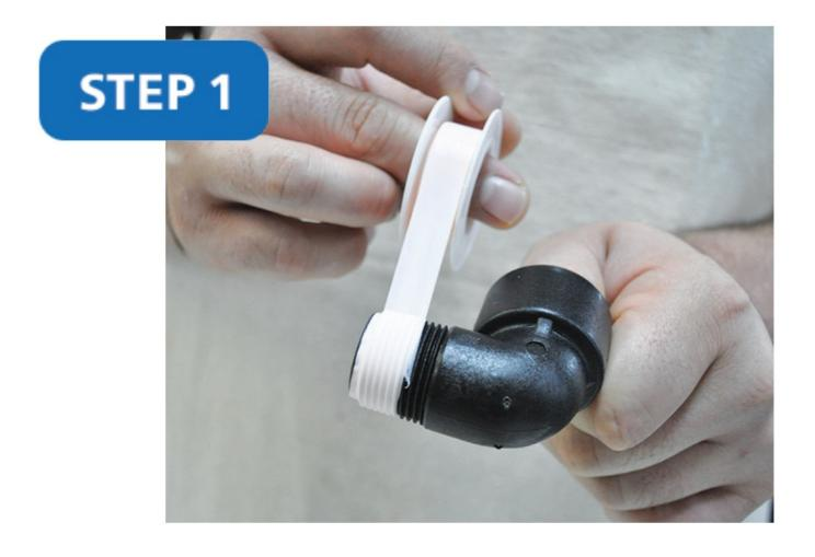
To begin, be sure to wrap all pieces with the thread seal tape, in a clockwise rotation, around the pipe threads. This will prevent the tape from coming off during assembly.
