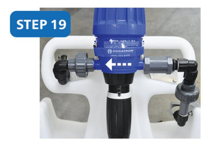
Install the unit and assemblies onto the cart, with the inlet side on the right side of the cart. The Dosatron arrow will be pointing left.
