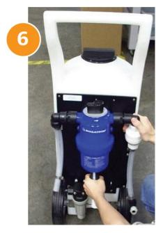
7. Insert the hose onto the filter barb and secure with the clamp.
