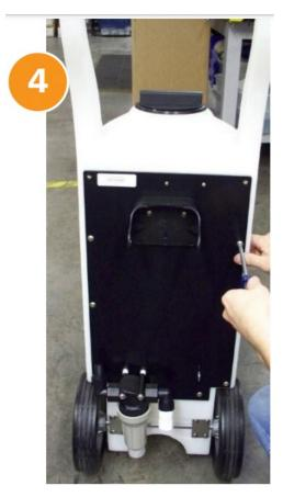
5. Using the instructions included, assemble the Quick Hook-up kit with the 20 GPM unit.
