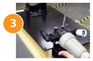
4. Re-attach the black plate back onto the Dosa Cart by installing eight screws around the plate except for the top two screws (these will be used for the crash bar, see step 9)
