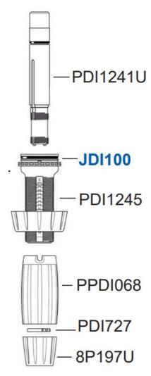
From the injection stem (PDI1241U), unscrew the upper insert (PDI1240U). Flip the stem (PDI1241U) upside down so the upper insert o-ring (20J006) comes off, discard and replace. Remove and replace the injection stem o-ring (JDI120) as well. Screw the upper insert back on.
