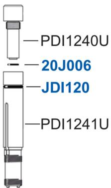
5. Slide the injection stem (PDI1241U) down into the sleeve (PDI1245), making sure the small key inside the sleeve is aligned with the longest groove on the white stem. Holding the graduated sleeve, pull down on the white stem as far as it will go. Thread the adjusting nut (PPDI068) back onto the sleeve (PDI1245). Reinstall "C" clamp (PDI727) by gently sliding it over the threads at the bottom of the white stem. Rotate clampuntil it clicks into place. Screw locking nut (8P197U) back on.
