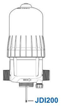
8. Carefully push the complete injection stem assembly in position at the bottom of the blue body, making sure desired scale is facing front of injector. Use a vertical motion to avoid bending the plunger. Keys at the top of the graduated sleeve should slide into the slots at the bottom of the body. Slide injection stem assembly nut (PDI702) up the sleeve and screw back on. Insert hose back onto the bottom of the check valve barb and screw hose nut (P150) back on.
