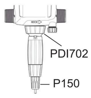
2. Unscrew check valve nut (8P168) and pull out check valve assembly (PJDI215). It may come out in one or two pieces. Be sure to remove the barb and check valve and discard.
