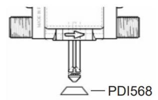
3. Hold the injection stem and unscrew the check valve barb (P169). Remove and discard the check valve seal (J051). If the seal isn't visible at the end of the injection stem, look inside the check valve barb. Carefully pry the check valve assembly (MPDI122) out of the injection stem and discard the assembly. Pay attention not to damage the lower end of the injection stem.
