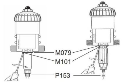
2. Pull the injection stem assembly down to expose the plunger. Remove the plunger seal (J009) and replace with new one.
