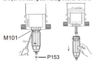
2. Pinch and remove the plunnger seal, then replace with the new one ( JDI211).
