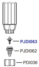
4. Replace the upper check valve (PJDI063) with the NEW one.
