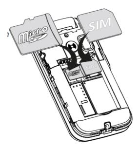
Insert the micro SIM or USIM card provided by the mobile service provider. Make sure that the SIM card's contacts are facing inwards and that the cut off corner is as shown. Should you need, but have problem to remove/replace the SIM card, use adhesive tape on the exposed part of the SIM card to pull it out.
