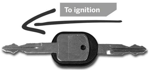
**NOTE:** After Step 3, move original key at least one foot from the vehicle to avoid causing a programming failure.
