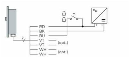
When in Fail Safe configuration, applying positive voltage to the control wire triggers the SL30SGL to lock (active-high locking signal). In the event of a power cut, the SL30SGL will unlock.
