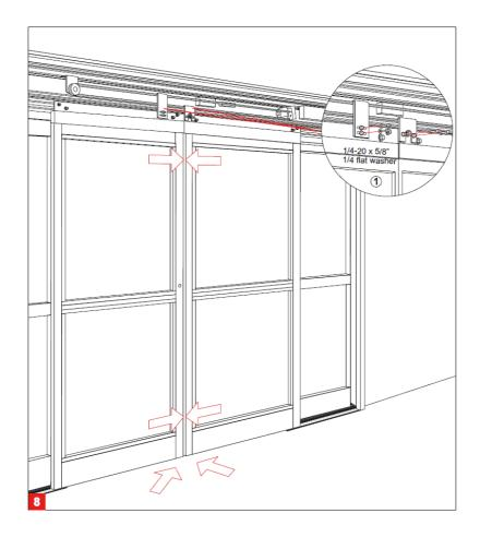
"SX" Panel Centerline Adjustment & "SO" Bottom Latch Installation
