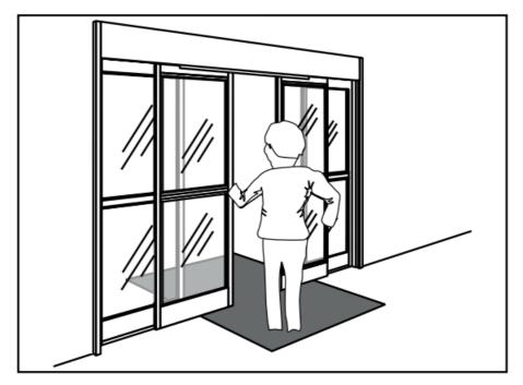
7. Step through the doorway onto the mat on the other side. The door should remain fully open without interruption.
