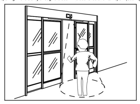
**NOTE:** If your door is set up for one-way traffic, the detector on the side not intended for use should be active until the door is within 6 inches of fully closed. The sensor should reopen the closing door if an object is detected a minimum of 24 inches from the door.
