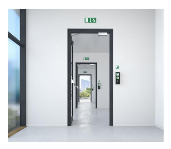
This type of system allows doors secured with an electrically operated lock, such as a keycard based access control system, to be used as an escape route door as it provides a way for the user to release the door efficiently in an emergency.
