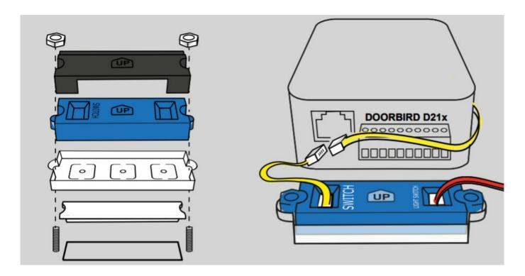
Make sure that the light switch is aligned upwards according to the "UP" marking and surrounded by the silicone seal.
