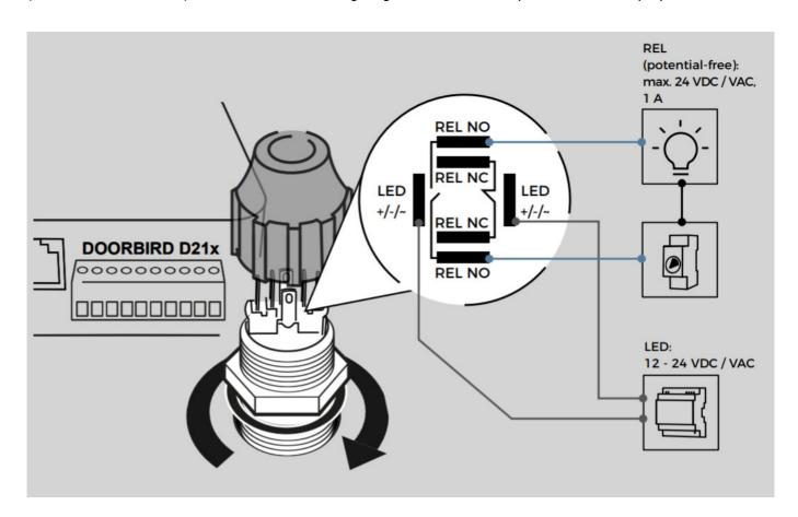
The round light switch provides a connection for the power supply of the integrated LED of the button (12-24 VDC / VAC) and an open/closed potential-free contact, which can be used e.g. for the control of a time relay (max. 24 VDC / VAC, 1 A) to switch the staircase lighting.
