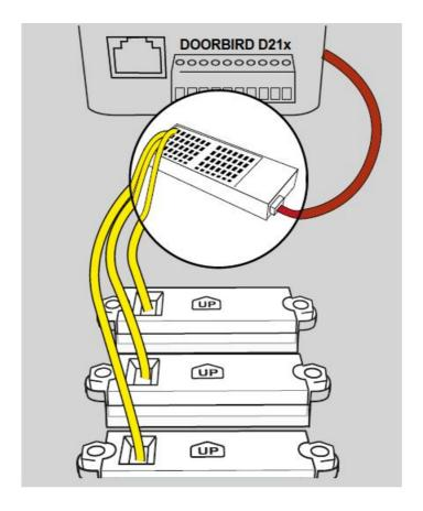
For door stations with several call buttons, the individual call buttons are connected to the ports of the Multi-Tenant Module using the yellow cable.
