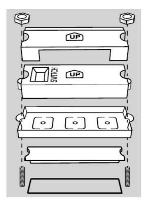
Make sure that the call button module is pointing upward according to the "UP" mark and is encased by the silicone seal.
