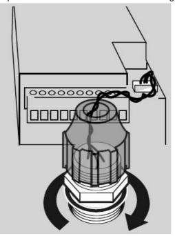
For the round call button, make sure that the sealing rubber is seated between the front panel and the nut.
