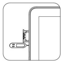
Take out the card slot and place the Nano card or Nano card and TF card with the metal side facing down.
