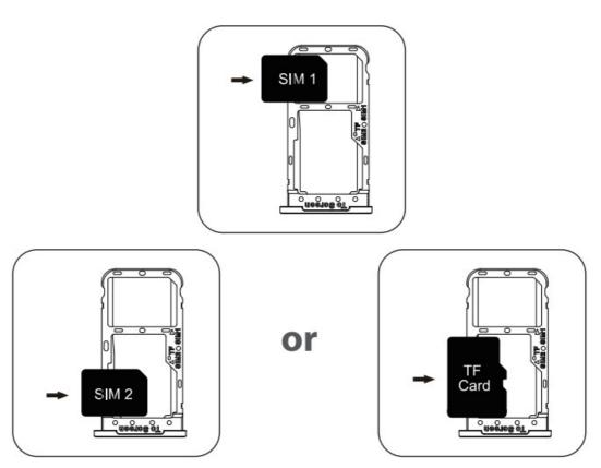
• With the pad facing up, insert the card holder into the pad in the direction of the arrow.
