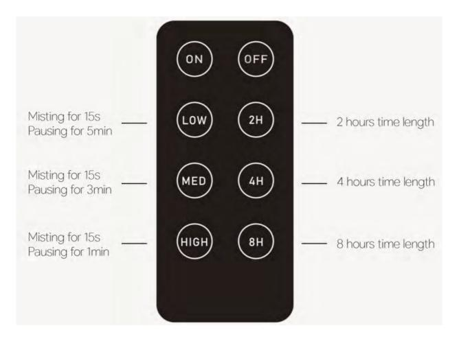
**Matching method**: Within 5 seconds of powering on the machine, press any key on the remote control, and the machine indicator light will flash, indicating successful matching.
