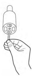
• **Tip**: If you are having difficulty seeing the tube holder inside the nozzle, hold a flashlight into the nozzle to increase visibility.
