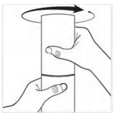
• Remove the empty oil bottle from the diffuser by turning it clockwise. Save this to use in the cleaning process of your diffuser.
