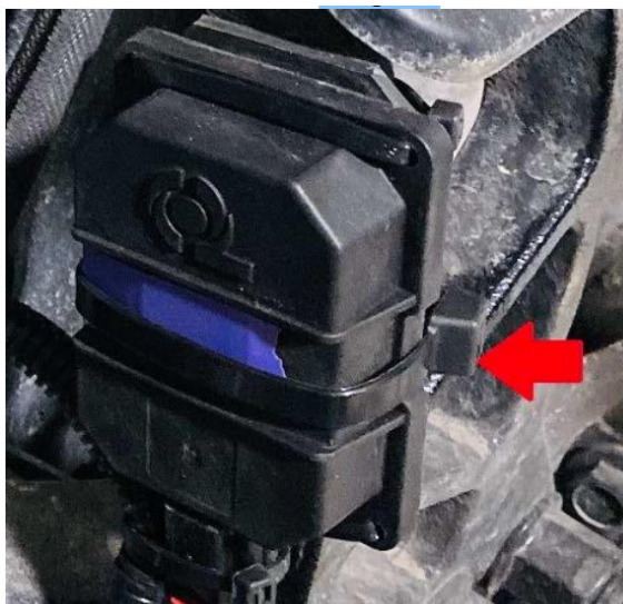
d. The holes at the four corners can be used for tie straps or bolts.
