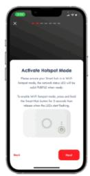
Enable Hotspot – hold down the Hub button for 5 seconds, release when the LEDs flash, wait for the button to have a solid purple light. Click on "Next"
