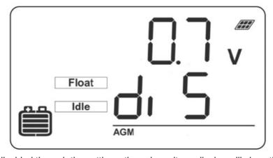
• When the charging is disabled through the settings, the solar voltage display will show the following menu display to indicate this was set intentionally by the user.
