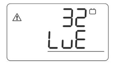
If a battery is still not detected after the fifth trial, the controller shows error number 32 to indicate this failure. The controller gives up until it is either manually reset by disconnecting and reconnecting solar power. The solar controller will not engage in this process if a new day is detected through the solar panel(s). Pressing the back button will also stop the process.
