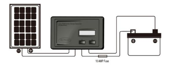
**NOTE:** The controller will not work unless there is a battery connected to the Battery 1 terminals.
