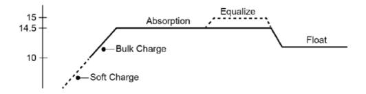
**Auto Equalize:** The GP-PWM-10-SQ has an automatic equalize feature that will charge and recondition your batteries once a month at a higher voltage to ensure that any excess sulfation is removed. This feature is recommended for Flooded batteries only. Check with your battery manufacturer.
