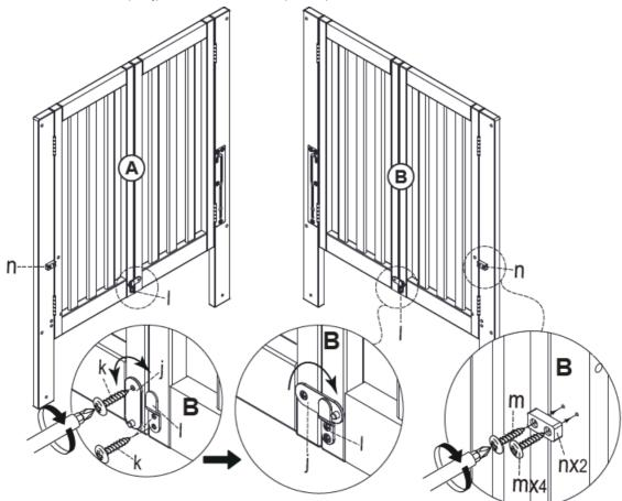
• Step 2: Connect the rail (C) and stabilizer bar (D) to the headboard (A & B) using the 5/8 screw (k). Assemble the plastic block (n) horizontally to the headboard (A & B) using a 3/4 screw (m). Do not fully tighten the bolts.
