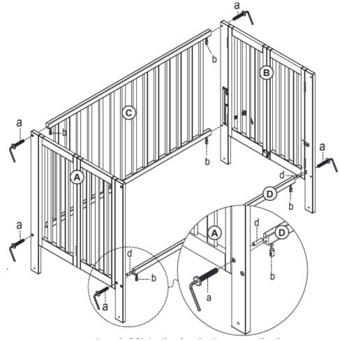
• Step 3: Slot in the metal pin into the notch of the left and right headboard side corner posts. Move it up and down to the highest level.
