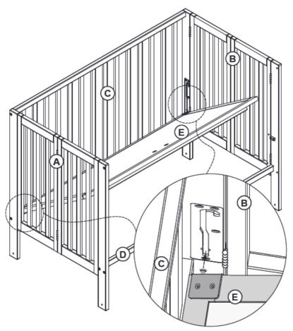
• Step 4: Connect the rail (C) to the headboard (A & B) using screws (a), nuts (b), washer (g), and washer (h).
