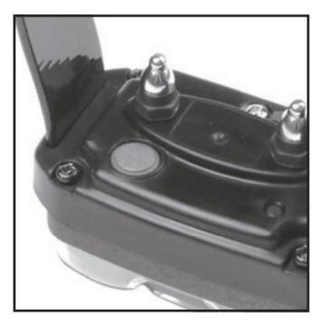
4. While the green LED is rapidly blinking on the receiver, press the button on the transmitter of the color you would like to code the receiver to. The LED light on the receiver will blink every 4 seconds when coding is complete.
