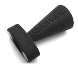
The microphone is provided (optional) with a magnetic cone that makes the microphone more directional. The cone can be easily removed by pulling it from the tip making the microphone omnidirectional, moreover, the cone provides protection to the sensor.
