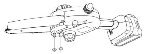
5. Turn the knob on the guide plate cover clockwise, pull the chain down when you turn the knob, and it can rebound quickly when you loosen the chain.
