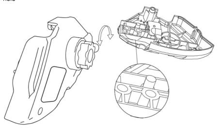
4. Align the convex points of the adjusting screws on the guide plate cover with the guide plate holes to install the guide plate cover.
