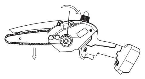
6. Use a socket wrench to tighten the outer hexagonal nut, and then screw the screw into the hole of the guide plate cover.
