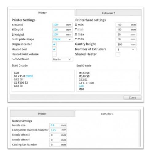
To CURA, this is simply a 1 nozzle printer that prints in the same colour. All the colour mixing options are done by the printer, not by CURA.
