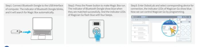
Note: Click the Key button of Bluetooth Dongle, and the corresponding Magic Box will sound a beep to facilitate users to find the corresponding connected device; long press the Key button of Bluetooth Dongle, and the Bluetooth Dongle will research a Magic Box.
