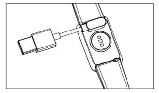
Note: Charge the watch to activate it before first use. The original power adapter must be used for charging.
