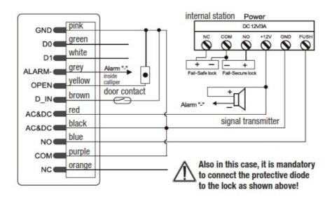
fail-safe lock: electric door opener or fail-safe lock
