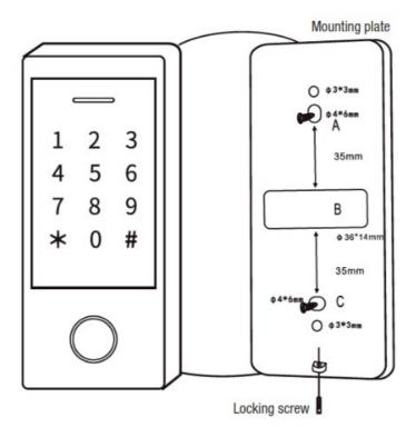
When choosing the installation site, make sure that the mounting plate lies tight and flat on its supporting surface while making contact with all four corners. Otherwise, acts of sabotage can be facilitated, and faulty activations of the sabotage alarm due to unwanted incidence of light into the device are possible.
