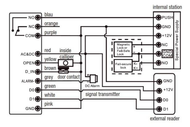
Also in this case, it is mandatory to connect the protective diode to the door opener as shown in chapter 4 (wiring instructions)!
