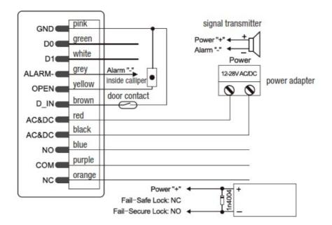
fail-safe lock: electric door opener or fail safe lock
