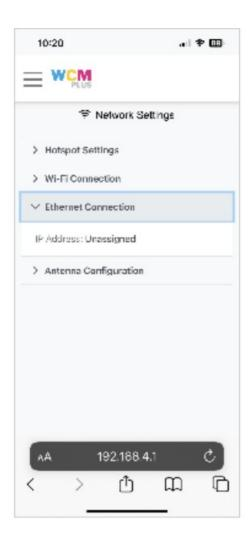
Antenna Configuration – Antenna configuration allows you to switch the antenna that is used for the hotspot and the antenna that is used for Wi-Fi. There are several benefits to this feature.
