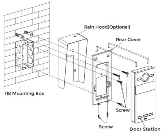
Product size:  $88 \times 188 \times 32.5$  mm Surface Mounting size:  $88 \times 188 \times 34$  mm
