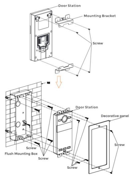
Product size:  $88 \times 188 \times 32.5$  mm Flush Mounting size:  $120 \times 230 \times 48$  mm Hole-cutting size:  $98 \times 219 \times 42$  mm
