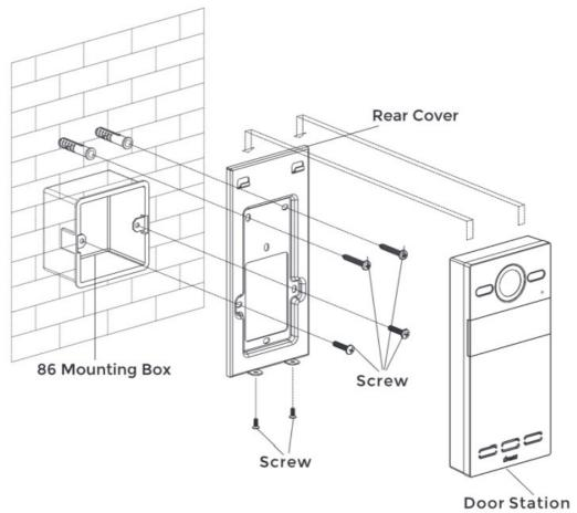
Product size:  $88 \times 188 \times 32.5$  mm Surface Mounting size:  $88 \times 188 \times 34$  mm Surface Mounting-118 Mounting Box
