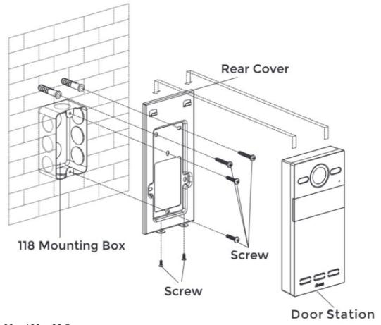
Product size:  $88 \times 188 \times 32.5$  mm Surface Mounting size:  $88 \times 188 \times 34$  mm
