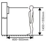
The camera should be 1450~1550mm above the ground. The camera at this height can capture human face perfectly.
