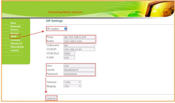
• Step 4: Go to the **Main** page to check if SIP is OK or not. If SIP is OK, then Outdoor Station is ready. If SIP is ERR, please make sure numbers are all correctly filled.
