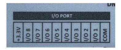
Note earlier production units have incorrect I/O Port labelling where I/O 1-8 are flipped 8-1. The above image shows the incorrect label.
