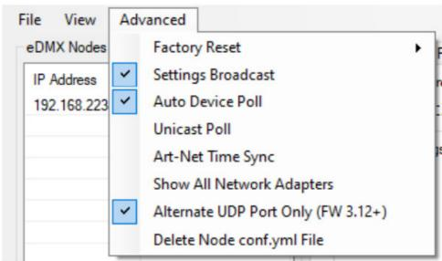
eDMX Node configuration can be saved/loaded from a simple Key:Value YML file. Select the node and perform Load/Save accessible in the File menu. Configuration files can be loaded from a file named "conf.yml" on the SD card however updates made to configuration are not currently saved by the node back to the conf.yml file. This is intended as a deployment mechanism where complete device configuration and show content can be prepared externally on an SD card.
