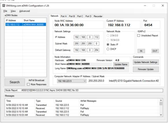
eDMX Configuration can find and configure eDMX MAX hardware on different IP subnets from the computer network adapter. There are some functions such as the Recorder that require both devices on the same IP subnet range e.g., Computer IP 192.168.0.100 Subnet 255.255.255.0 Gateway 192.168.0.254 when eDMX MAX is on default IP.
