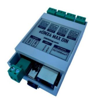
Network 10/100Mbps RJ45 socket. Pluggable 2way 5mm pitch terminal block for 7-28Vdc power input. Four 3way 3.5mm pitch pluggable terminal block connectors for DMX512.
