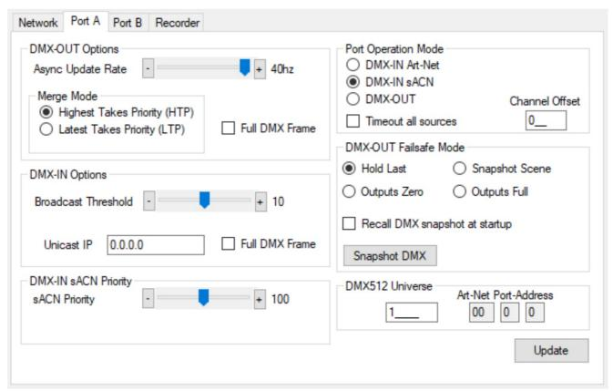
DMX512 ports can be individually configured as either DMX-OUT, with automatic dual sACN/Art-Net protocol support, or DMXIN, with manually selected sACN or Art-Net protocol. When configured as DMX-IN a single Unicast IP address destination may be specified but in the majority of applications leaving this field at 0.0.0.0 is appropriate.
