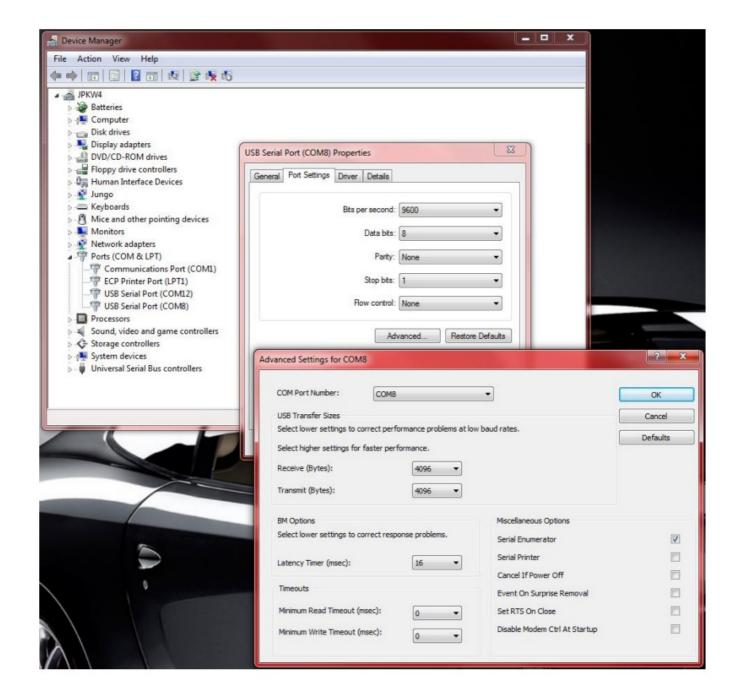
On occasion, you may wish to change the COM port number an eDMX2 PRO unit has been assigned by Windows. This can be done through the Device Manager applet by right clicking on the USB Serial Port of interest (unplug/re-plug the unit and observe if unsure which COM port) then select properties, Port Settings tab, Advanced button and finally choose the desired COM Port Number.
