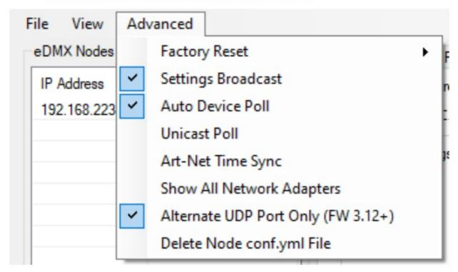
**IMPORTANT**: Firmware v3.11 and older. Once you've finished configuring your eDMX product close the configuration utility before starting your lighting control application if it's running from the same computer. From eDMX Configuration v1.24+ an eDMX Node configuration can be saved/loaded from a simple Key: Value YML file. Select the node and perform Load/Save accessible in the File menu. Firmware v3.12+ can load configuration from a file named "conf.yml" off the SD card.
