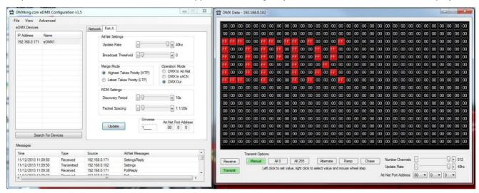
The DMX Display utility works with any manufacturers Art-Net hardware and can be useful for diagnostics and simple testing of DMX512 fixtures.
