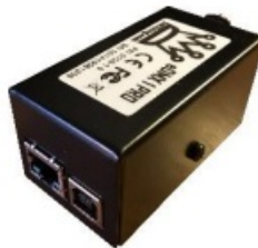
USB type B power socket + Ethernet RJ45 socket
