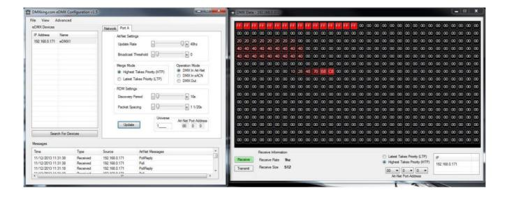
The DMX Display utility works with any manufacturers Art-Net hardware and can be useful for diagnostics and simple testing of DMX512 fixtures.
