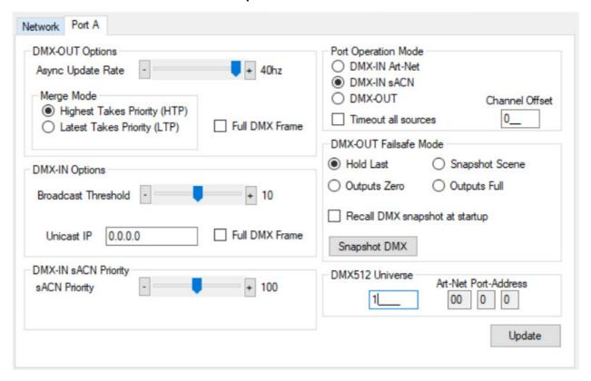
DMX512 ports can be individually configured as either DMX-OUT, with automatic dual sACN/Art-Net protocol support, or DMXIN, with manually selected sACN or Art- Net protocol.
