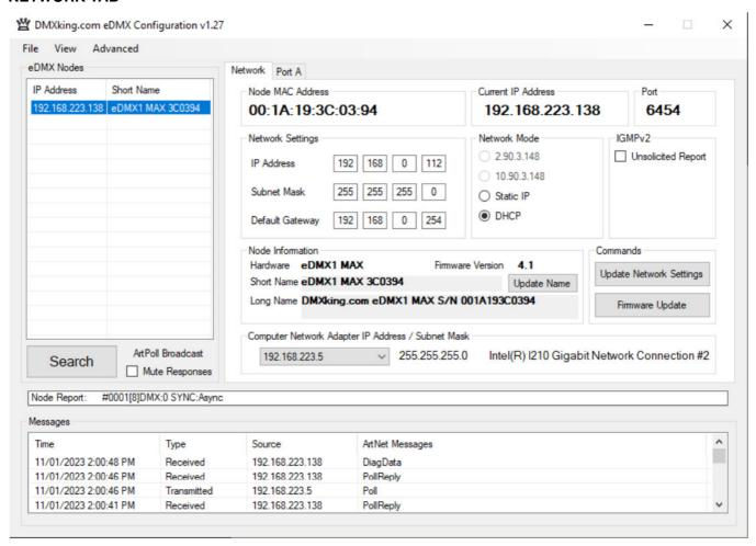
eDMX Configuration can find and configure eDMX MAX hardware on different IP subnets from the computer network adapter.
