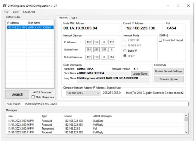
eDMX Configuration can find and configure eDMX MAX hardware on different IP subnets from the computer network adapter. There are some functions such as the Recorder that require both devices on the same IP subnet range e.g., Computer IP 192.168.0.100 Subnet 255.255.255.0 Gateway 192.168.0.254 when eDMX MAX is on default IP.
