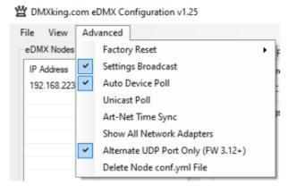
eDMX Node configuration can be saved/loaded from a simple Key:Value YML file. Select the node and perform Load/Save accessible in the File menu.
