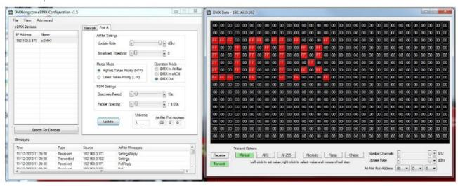
Changing to Receive mode will display the selected Art-Net universe number with merged streams if more than 1 is present. Note Art-Net II unicast is not supported meaning only Art-Net broadcast streams are displayed.
