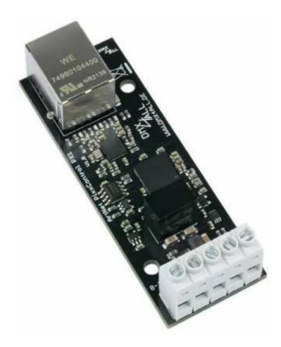
The ArtNet PixxControl PX1 is a compact ArtNet (DMX over Ethernet) interface, designed to convert ArtNet into an independent control signal for multiple digital LEDs.
