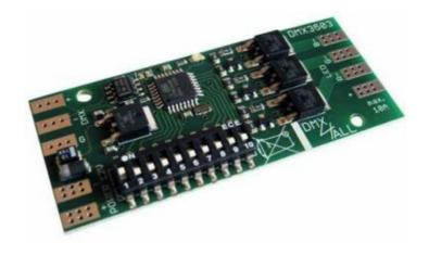
The DMX-LED-Dimmer MaxiRGB is a device designed for driving RGB LED strips with 12V or 24V. It features 3 separate LED outputs that can be independently controlled via DMX. These outputs can be used for RGB or separate single color LED strips. Additionally, the device has internal color gradients that can be called without external control. The operating voltage of the DMX-LED-Dimmer MaxiRGB is also the operating voltage of the LED strips.
