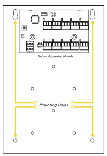
The X1 Output Module (X1-OUT-EXP) has a 1 through 9 addressable rotary dial that is factory defaulted to 1. Additional output modules need to be addressed in sequence.
